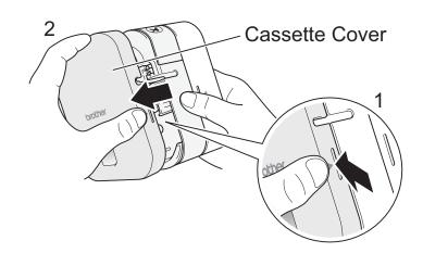
Insert the Tape Cassette following the drawing marked inside the case. Confirm that the tape is aimed at the green Tape Outlet and gently press the Tape Cassette into your machine until it locks into place.
