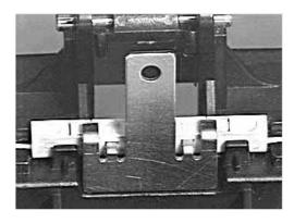
**5.3** Slide the bottom of the cap lifter inward until it is in a vertical position, lifting the splice slightly out of the cradle.
