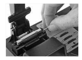
**4.3** Gently continue pushing the fiber into the splice until resistance is felt. When fully inserted, the first fiber should be straight or have a slight bow – up to .1 inch (3 mm).
