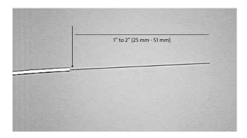
**3.3** Clean the bare glass by pulling the fiber through an alcohol soaked lint-free wipe. This will remove any fragments or dirt remaining on the fiber.
