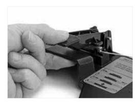
**4.10** Remove the Fibrlok Splice from the assembly tool by first removing the fibers from the foam retention pads and then lifting the splice from the splice holding cradle.
