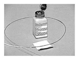
**2.3** Remove the Fibrlok® Splice from protective package. Load the splice into the assembly tool by pressing firmly at the ends of the splice.
