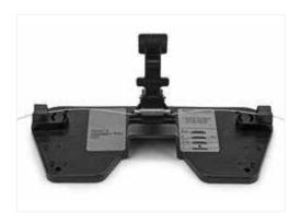
**4.8** Push the first fiber back against the second fiber until there are equal bows in both fibers.
