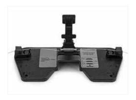
**4.9** Pivot the handle of the Fibrlok\* Assembly Tool 2501 down until it contacts the cap of the Fibrlok splice. Squeeze the handle of the assembly tool as shown in order to close cap and actuate the splice. When possible, secure the tool to a work surface for added support. A snap sound will be heard when the splice is actuated.
