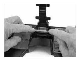
**2.4** If using the Fibrlok Assembly Tool 2501, rotate the toggle arms for the appropriate fiber size.
