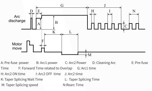
Diagram of ARC discharge condition
