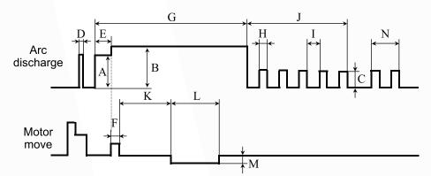
A: Pre-fuse power B: Arc1 power C: Arc2 Power D: Cleaning Arc E: Pre-fuse
